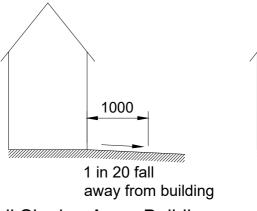
Provide A.G. drain or spoon drain to discharge into S.W.D. system
